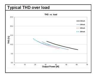
ELEMENT 60220-240350 D CS L Typical THD Vs Load
